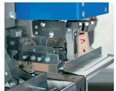
Starres (passives) Fingerschutzsystem Fixed (passive) finger guard system
