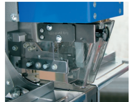
The attaching machine shown here is equipped with pucker-free attachment technology
